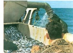
The catch operation is less time consuming with one-boat trawling. The fish pump reduces draining time considerably.
